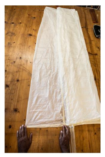
Put all the panets to the right side and fold over each panel from the right side onto left side like turning the pages in a book and pull the top of the opening outward..
