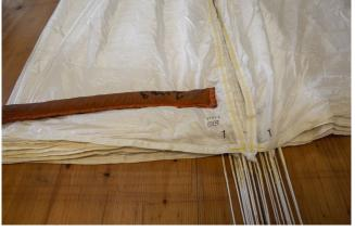
Put a packing weight for fixation on the last panel and than all the panel from the right side can be shifted to the that side.
