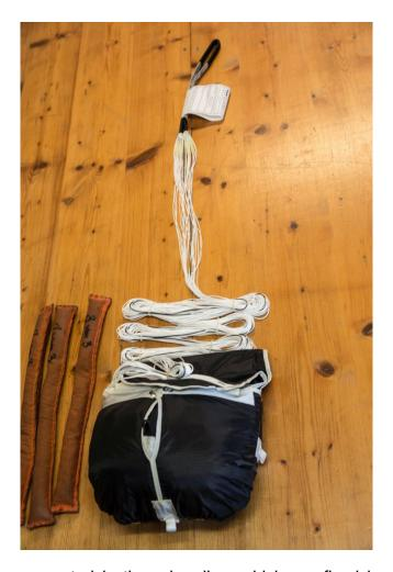
The suspension lines are sorted in three bundles, which are fixed by rubbers.
